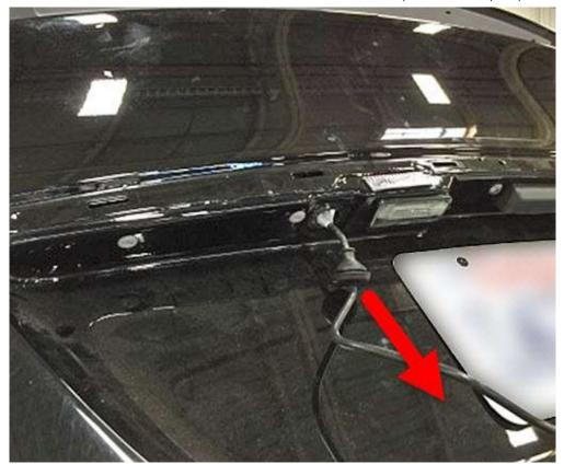
7. Release the screws (x2) that secure the camera to the liftgate applique bracket (torque 2.8 Nm
